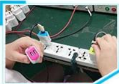
9. Aging test for travel charger
